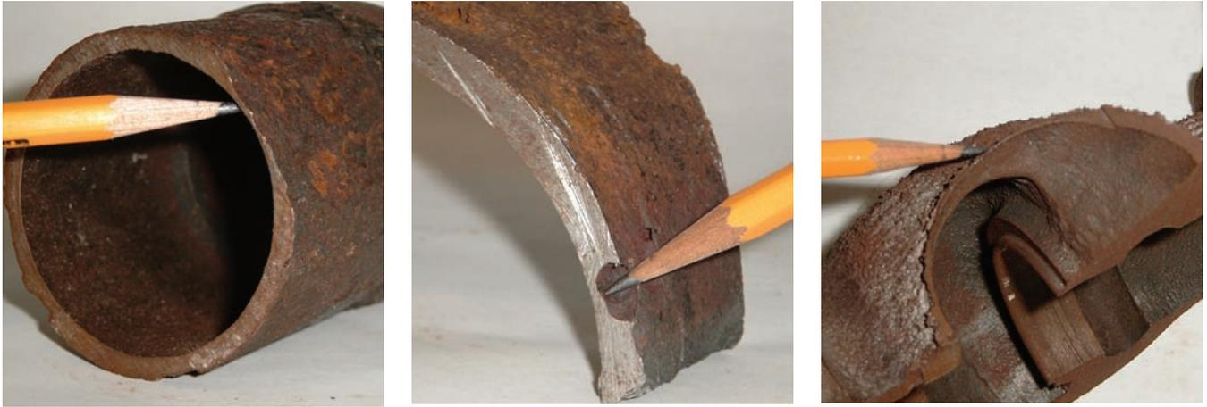
**Photo 1 (left):** Uniform corrosion on the exterior of refrigerant piping. **Photo 2 (center):** Pitting corrosion on the exterior of refrigerant piping. **Photo 3 (right):** Erosion on the inside of a valve due to change in direction of a two-phase refrigerant.
