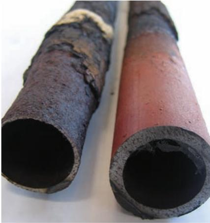
*Photo 6: This pipe carried subcooled, high-pressure liquid ammonia. At installation, only the portion of pipe on the right was painted. When the insulation became saturated with water, corrosion reduced the pipe on the left to one-sixth its original thickness while the painted pipe suffered little damage.*
