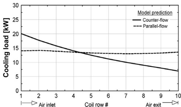
Fig. 11. Cooling capacity across the evaporator for the counter-flow and parallel-flow configurations.
