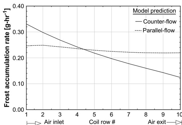
Fig. 14. Comparison of the frost accumulation rate at each row predicted by the counter-flow frost model and the parallel-flow frost model after 1h of operation.
