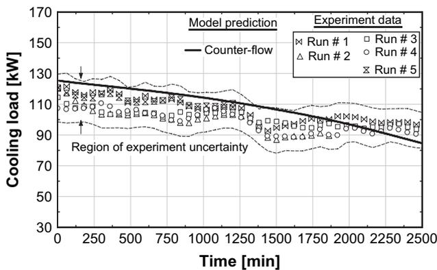
Fig. 7. Comparison of the evaporator cooling capacity measured during the experiment and the evaporator cooling capacity predicted by the counter-flow frost model over time.
