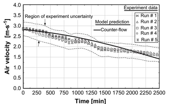
Fig. 5. Comparison between the average face velocity of the evaporator coil measured in the experiment and the face velocity predicted by the counter-flow frost model over time.
