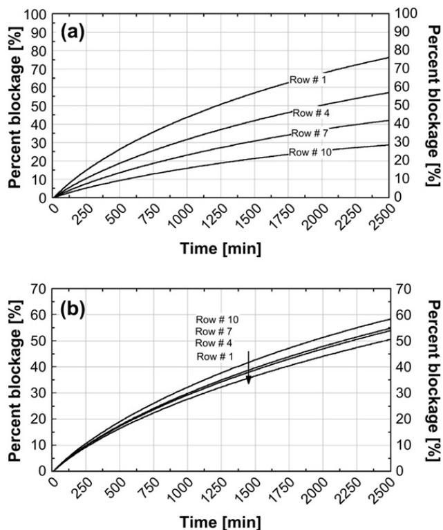
Fig. 15. Percent blockage of the air path caused by frost accumulation at different rows of the evaporator coil over time for (a) counter-flow and (b) parallel-flow circuiting.
