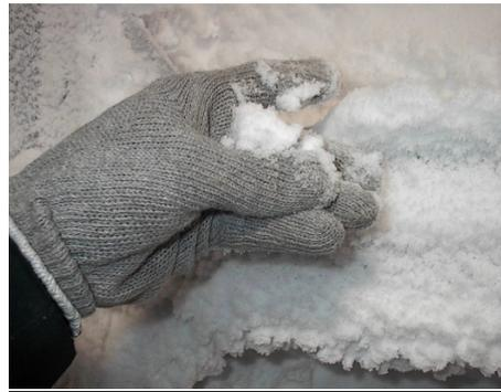
Figure 5: Low density frost forming on an evaporator due to high coil TD and presence of supersaturated air.
